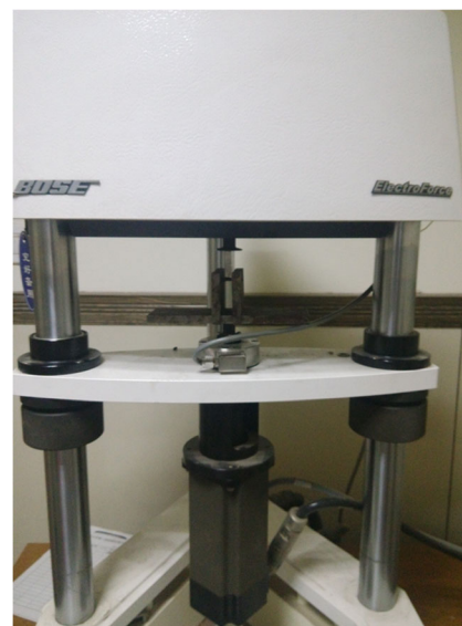
Fig. 1 The rat tibia or femur was horizontally positioned on the fixture of the machine. The compression was located in the center of whole tibia and applied in the sagittal plane
